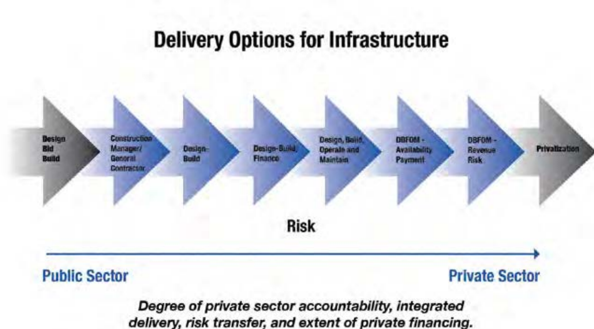
Figure 4-1 Delivery Models for Public Infrastructure and Other Public Projects Source: Association for the Improvement of American Infrastructure
